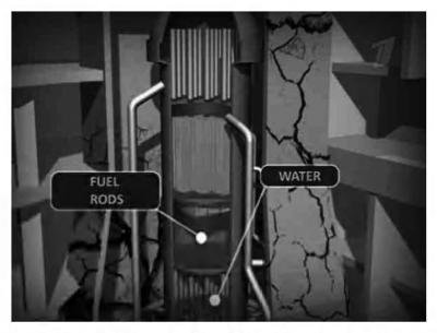
The cross-section drawing of damaged pressurised zone of unit #2
